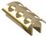
The riders have a standard length of 50 mm and are cut according to the available space. To guarantee optimum adhesion, it is recommended not to reduce the riders below the minimum length of 8 mm.
